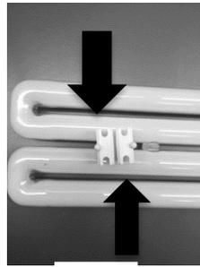
6. Insert the new bulb into its socket, on an angle (about 20°) **(e)**, then gently push the bulb backward until it rests against the back of the unit with the clip securing it into place **(g)**.
