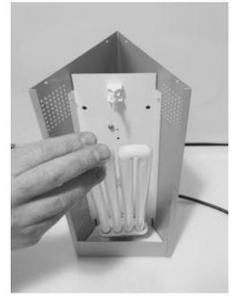
4. Lift the old fluorescent tube out of the unit and carefully dispose of it. If it has been broken, carefully clean the interior of the unit to remove any glass fragments that may have come loose.
